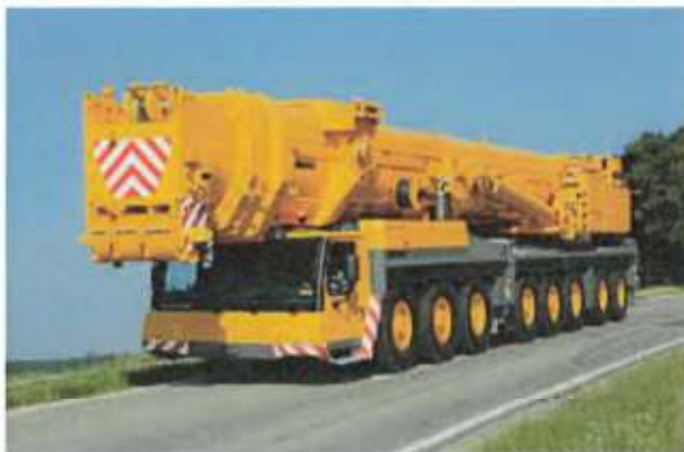
Plate 3.5: Crane for Wind Turbine Erection 7
